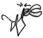
4. Use pliers to bend the tip of each side slightly, away from the middle of the hanger. This keeps the rubber band from slipping off so easily.
