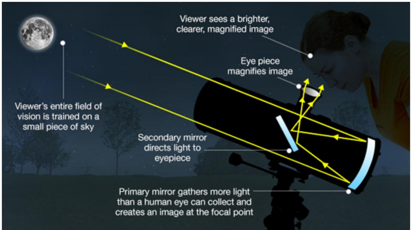
Another benefit of using mirrors instead of lenses is that big mirrors are easier and cheaper to make than big lenses. Reflecting telescopes can be much larger and therefore look deeper into space.
