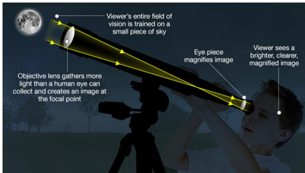
A telescope's ability to collect light depends on the size of the objective lens, which is used to gather and focus light from a narrow region of sky.
