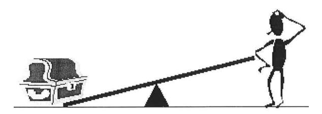
With the lever, you can push instead of pull. The lever will make the chest feel like it has less *weight*. The weight of the chest isn't really less. The simple machine lets you use a smaller force over a greater *distance* to lift the chest.
