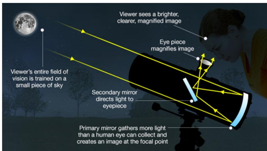
Another benefit of using mirrors instead of lenses is that big mirrors are easier and cheaper to make than big lenses. Reflecting telescopes can be much larger and therefore look deeper into space.
